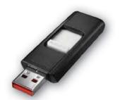
USB Data Sharing – Make room on the tool belt for a flash drive as the USB data sharing port has become another important device to have in commissioning (upload/download settings from one boiler to the next), servicing (download data and email file to factory for assistance) and analyzing boiler operation (historical info can be downloaded & saved in .CRV formatted files).
